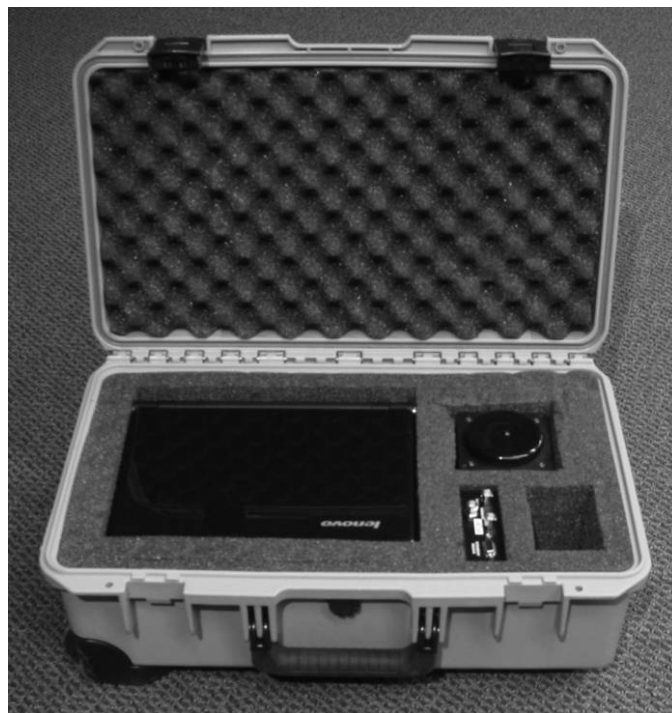
FIG. 2.—A complete PICO system in its case. Cables and power supplies (not visible) are stored beneath the laptop computer at left. The camera is stored at upper right. The GPS timing system is stored at lower right. The empty recess at far lower right provides storage space for camera mounting hardware and other accessories. Wheels (at left) and a retractable towing handle (at right, not visible) reduce observer fatigue during travel.
